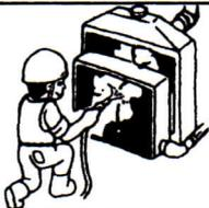
An illustration showing a worker in a hard hat and safety vest using a tool to clean the radiator of a piece of machinery.
